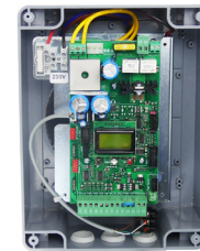
USER-1 24V DG MAXI Controller with built in transform- er housed in an external enclo- sure for 24V slide gate operators.
