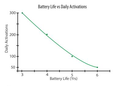
Note: Battery life is dependant on many factors, including daily activations, time used per activation, radar range and external conditions.
