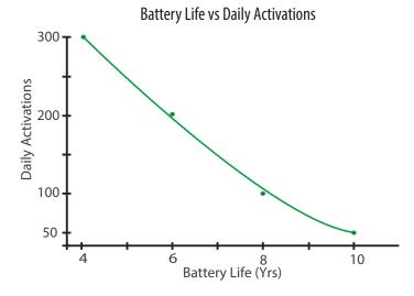
Note: Battery life is dependant on many factors, including daily activations, time used per activation, radar range and external conditions.
