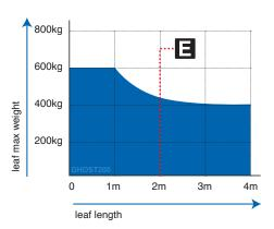
If the leaf length is bigger than 2m or if you use reversible models you must install the electric-lock to block the gate in closed position. The height and the leaf structure, as well as the presence of strong wind, can cause the reduction of the value of the data contained in table or make it necessary to use an electric lock also for leafs shorter than 2m.
