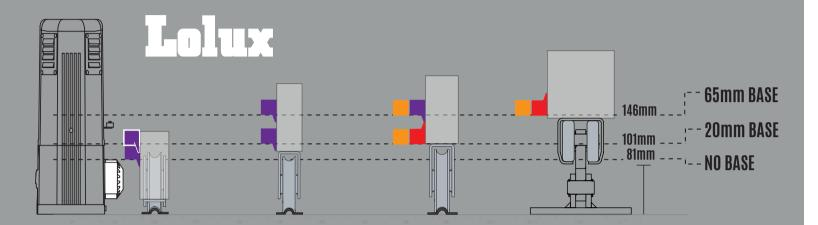
RECESSED WHEEL 90mm (300550) Wheel Rating: 300kg Bottom Channel: 100x50 Rack: AR-6FPNR BOTTOM MOUNT WHEEL 80mm (327-80S) Wheel Rating: 200kg Bottom Channel: 100x50
