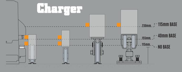
**RECESSED WHEEL:** 160mm (338-160) Wheel Rating: 600kg Bottom Channel: 150x50 Bottom Channel: 100x50 Rack: AR-STERHOL12
